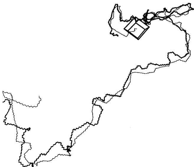
Fig. 5.12 Comparison of the chain structure for one sample before (thin line) and after (thick line) heat treatment. Only the coordinates of the continuous primary chain have been shown. The molecular dynamics “unit cell” which is filled by images of the primary chain, is also shown.
