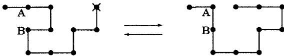
Fig. 2.6 The kink-end reptation ( \rightarrow ) and end-kink reptation ( \leftarrow ) moves. In \rightarrow , a kink has been cleaved from AB and two new steps have been attached at the end marked with a cross. Note that the new end steps are permitted to occupy one or both of the sites abandoned by the kink.
