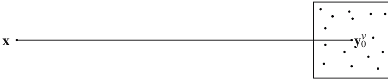
Fig. 8.1. Interaction of a particle at \mathbf{x} with a set of particles in \Omega_\nu^{\text{far}} around the center \mathbf{y}_0^\nu .
