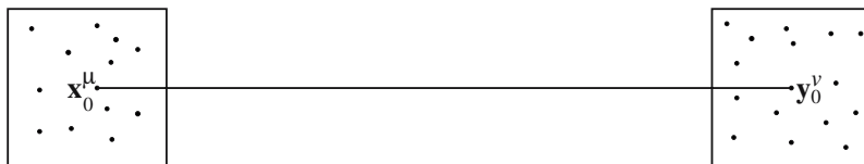
Fig. 8.35. Interaction of a cluster of particles around the center \mathbf{x}_0^\mu with the particles from a distant cluster of particles around the center \mathbf{y}_0^\nu .
