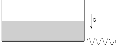
Fig. 3.25. Configuration for the simulation of surface waves in granular media: The lower wall oscillates with a given frequency f .
