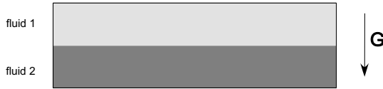
Fig. 3.18. Initial configuration for the Rayleigh-Taylor instability; the heavy fluid sits on top of the light fluid.
