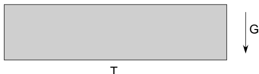
Fig. 3.22. Rayleigh-Bénard convection, configuration with heated lower wall.
